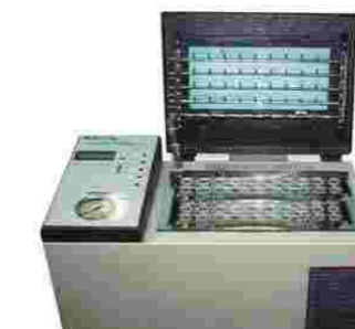
Nitrogen Concentrator / Evaporator
